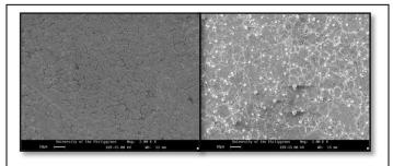
Fig. 2. SEM micrograph showing the surface of stainless steel and the overall feature of the randomly distributed silica particles on stainless steel substrate taken at 2000 X magnification
