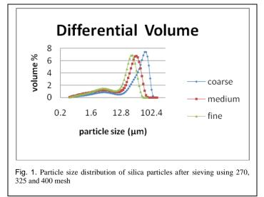
Industrial grade 98% purity silica powder from Dalisay Philippines Corporation was prepared by sieving the particles using 270, 325 and 400 meshes in a mechanical shaker prior to suspension preparation. Five grams (5g) of sample from each mesh were then analyzed using Coulter Counter to evaluate its particle sizes and distribution.
