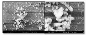
Fig. 3. Electrophoretically deposited silica on stainless steel substrate showing aggregated silica particles taken at 2,000 X and 10,000 X magnifications respectively.
